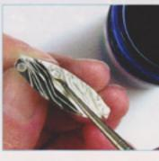
This type of texture works well with a patina. Liver of Sulphur mixed up quite strongly will give a black finish, which can be polished back from the high spots, discs and balls to reveal a good contrast. Platinol can also be used on a fine paintbrush down in the texture to blacken specific parts only. Alternatively, you can leave it silver and just burnish the high spots.
