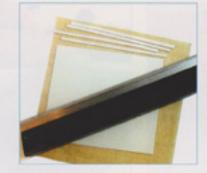
Place the PMC sheet on a clean, dry surface. Using a rigid straight tissue blade, cut out strips of the sheet approximately 2mm wide. The rigid blade pressed straight down onto the sheet will cleanly cut through and is more accurate than using a craft knife. If you do use a craft knife, use a steel ruler so you can cut a very straight line. Put the cut sheet aside.
