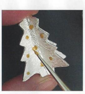
STEP 8 Polish using a tumble polisher or brass brush. Use a burnisher to shine up the edges of the trees. Dip in Liver of Sulphur if you like an antiqued look, and then polish the high spots of the texture to create a contrast and show up the branches. Using ceramic or glass paint, apply colour to the dips with a small paintbrush, dry and finish following the manufacturer's instructions.
